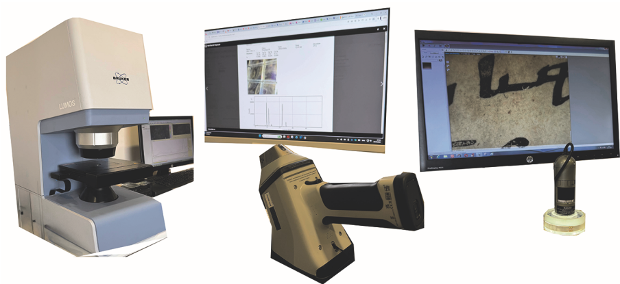
Pl. 1: FTIR-ATR Spectroscopy, XRF Spectroscopy and Dino-Lite Microscope setups
